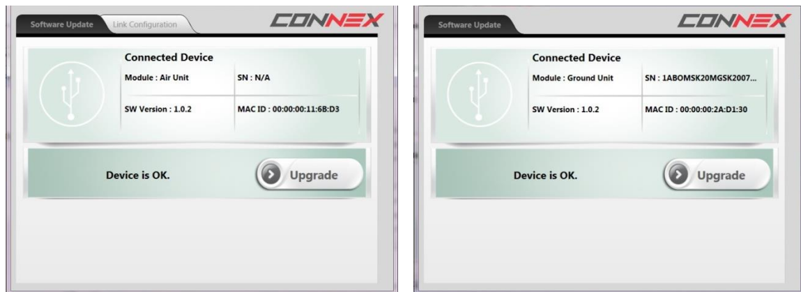
Figure 35: Upgrading the Air Unit (shown on left) or Ground Unit (shown on right)
