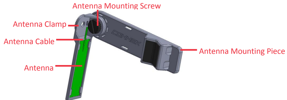
Figure 26: Air Unit Cable Antenna Mounting Accessory – With Flat Cable Antenna – Box 2
