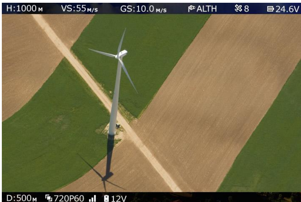
Figure 33: OSD View – with Telemetry Information
