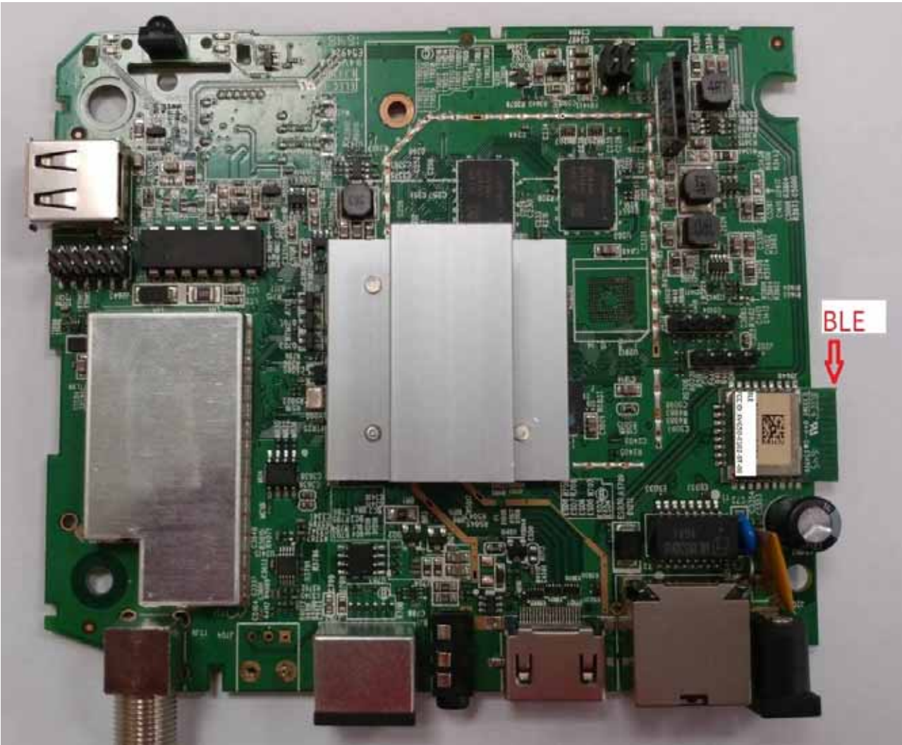
Module install location on Aria6/7.
