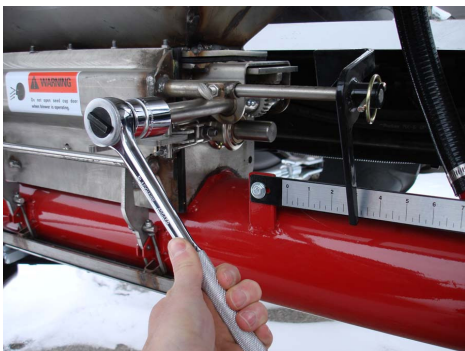
Adjusting the Meter Gate
