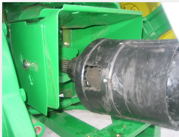
Figure 20: Attached PTO Driveline
