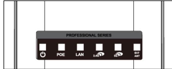
**2.4GHz Wireless Activity:** Blinks rapidly when 2.4GHz wireless data traffic is passing through the Pro Access Point.
