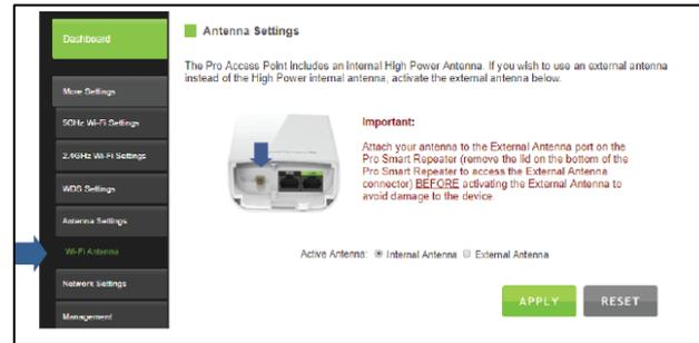
It is important that you attach the external antenna to the External Antenna Port **BEFORE** activating the External Antenna Port to avoid damage to the Pro Access Point.
