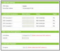
For WDS connections to work properly, the MAC address associations must also be configured on each individual WDS enabled Access Point, not just the one you are currently configuring. For example, if you are connecting three WDS-APs, AP 1 must have AP 2 and AP 3's MAC address conifgured, while AP 2 has AP 1's and AP 3's MAC, and AP 3 has AP 1's and AP 2's MAC configured. Every WDS connected device must also be using the same wireless channel as all other WDS connected devices.
