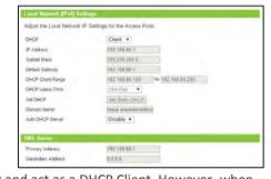
Note: If you choose to use a Static IP address for the Access Point, you will no longer be able to access the web menu using http://setup.ampedwireless.com. You must use the assigned IP address to access the web menu.
