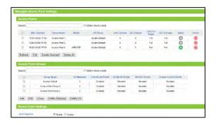
A **System Default Access Point Group** is available and will include all Managed Access Points if you have not yet configured any additional Access Point Groups. The System Default Group settings can be overridden when new Access Point Groups are created and additional Access Points are added to the new Groups and away from the System Default Group.
