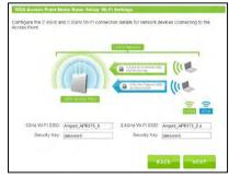
To change it, enter a new name in the SSID field. Users connecting wirelessly to the Access Point will use these IDs to identify your wireless network.
