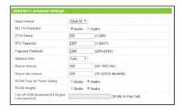
802.11n Protection: Increases reliability, but reduces bandwidth (Provides more bandwidth than 802.11g Protection).
