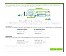
To change it, enter a new name in the SSID field. Users connecting wirelessly to the Access Point will use these IDs to identify your wireless network.
