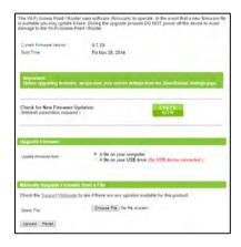
does not have access to the Internet, you can manually upgrade the firmware by downloading the firmware file from the Amped Wireless Elite Support website. The firmware update is downloaded as a zip file and you will need to have an unzipping program to open the file. Inside the file will be a text document with details on the current firmware release and instructions on how to upgrade the firmware.
