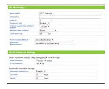
different VLAN ID. For example, if SSID 1 is assigned to VLAN 1 and SSID 2 is assigned to VLAN 2, then devices connected to SSID 1 will not be able to see or access devices or files on SSID 2 (VLAN 2). VLAN IDs can range between 1 and 4094.
