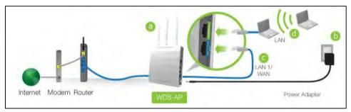
d) Connect an Ethernet cable between the Access Point's LAN2 port and your computer's network port or connect to the Access Point's Wi-Fi Network: Amped\_APR\_2.4 or Amped\_APR\_5.0, Password: wireless.
