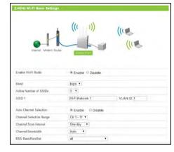
different name, VLAN assignment and security key. Additional SSIDs is sometimes referred to as Guest Networks.
