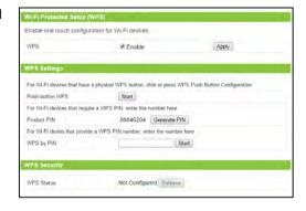
Option B: PIN: Some wireless devices use PIN number to access wireless network. If your wireless device requests for a PIN number, use the PIN code located here.
