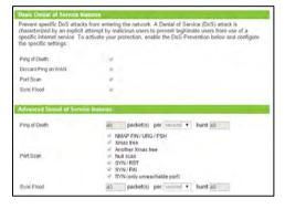
The Router can assist in preventing these types of attacks by scanning the network for patterns of activity that represent DoS attacks. If a pattern comes in frequently, the Router can attempt to block messages containing that pattern and thus protect the server from becoming overloaded and unresponsive.
