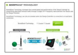
5GHz band is not available or becomes too weak, BoostBand Technology will automatically switch over to the 2.4GHz band.
