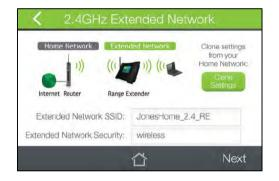
The SSID of the Extended Network will have a "\_RE" at the end of its name. For example: Home\_Network\_RE.
