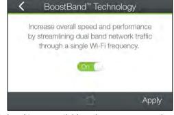
BoostBand Technology will use the faster, 5GHz band. If the 5GHz band is not available or becomes too weak, BoostBand Technology will automatically switch over to the 2.4GHz band.
