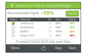
If you fail to find any Wi-Fi networks, or your signal strength is below 70%, the Range Extender may be placed too far from the Wi-Fi network that you are trying to extend. Move your Range Extender closer to the Wi-Fi network that you are trying to extend and tap Rescan to scan again.
