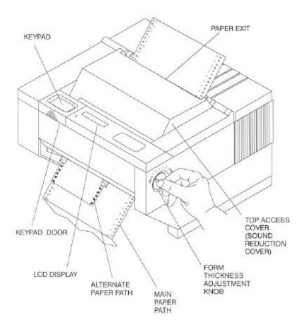
Figure 1-1: External Printer Parts (Dual Path and Sound Reduction Access Cover) (Sheet 2 of 2)
