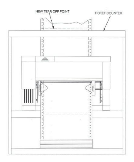
Figure 3-10: Printer Located Under Countertop
