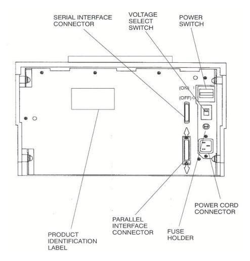
Figure 1-3: Back Printer Parts
