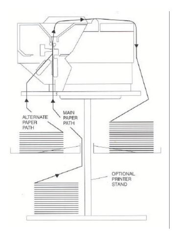
Figure 3-12: Main and Alternate Paper Paths (Cut Sheet not Shown)
