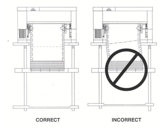
Figure 3-4: Placement of Continuous Forms
