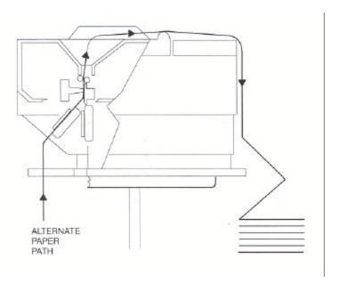
Figure 5-3: Alternate Tractor Path
