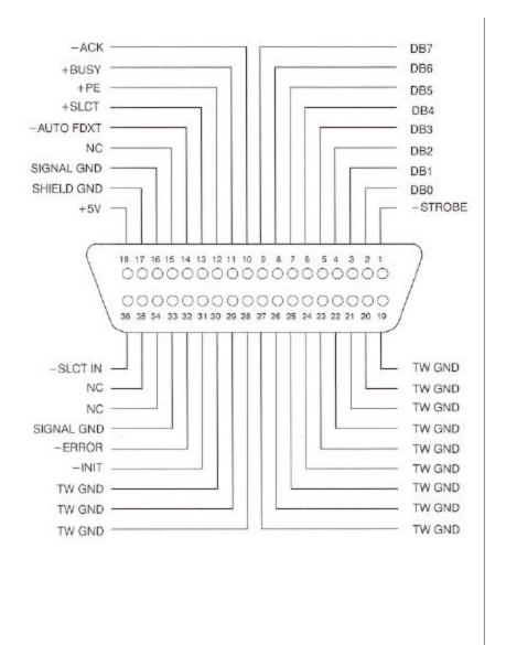
Figure B-1. 36 Pin Parallel Interface Connector
