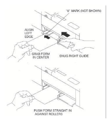
Figure 3-8: Loading Cut Form
