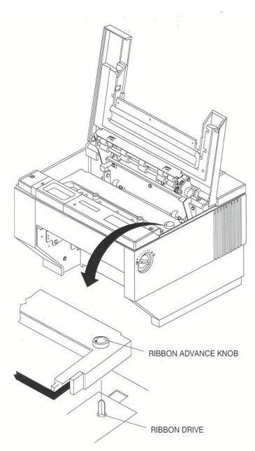
Figure 1-9: Install Ribbon Cartridge
