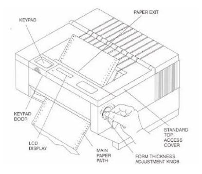
Figure 1-1: External Printer Parts (Standard Model) (Sheet 1 of 2)
