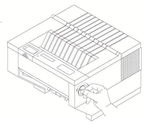
Figure 3-11: Manually Move Form Thickness Adjustment Knob
