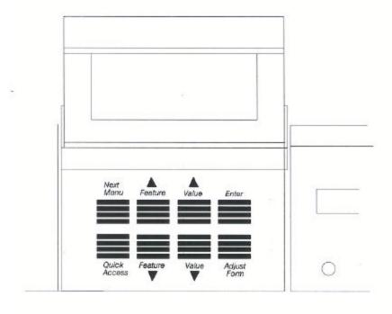
Figure 4-1: Setup Mode Keys
