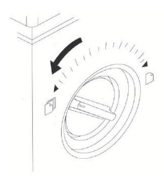
Figure 1-6: Form Thickness Adjustment Knob
