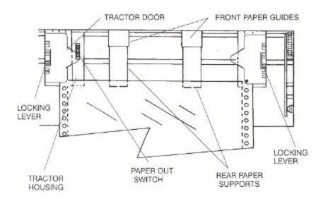
Figure 3-2: Load Paper In Tractors (Typical)
