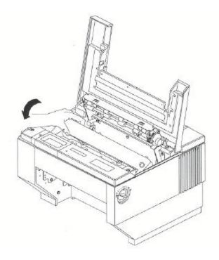
Figure 1-8: Position Ribbon Cartridge In Printer
