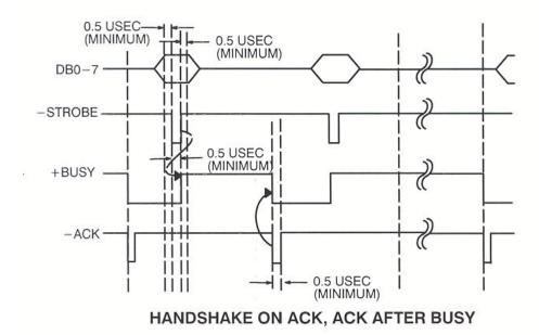
Figure B-2: Signal Timing Pattern (Sheet 1)
