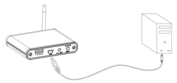
4. Manual Channel mode: set the dip switch "L" to upward side, 1-4 to downward side, receiver set to Manual channel mode, press the channel button, the channel will switch from 1 to 4, led show the current channel.
