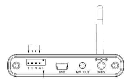
5. Loop Mode: set the dip switch "L" and 1-4 to downward side, the receiver set to Loop mode, the receiver will auto switch channels every 5 second from channel 1 to channel 4.
