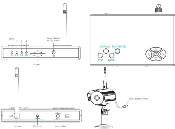
There are 10 keys and 1 switch on the receiver, one key on the camera.
