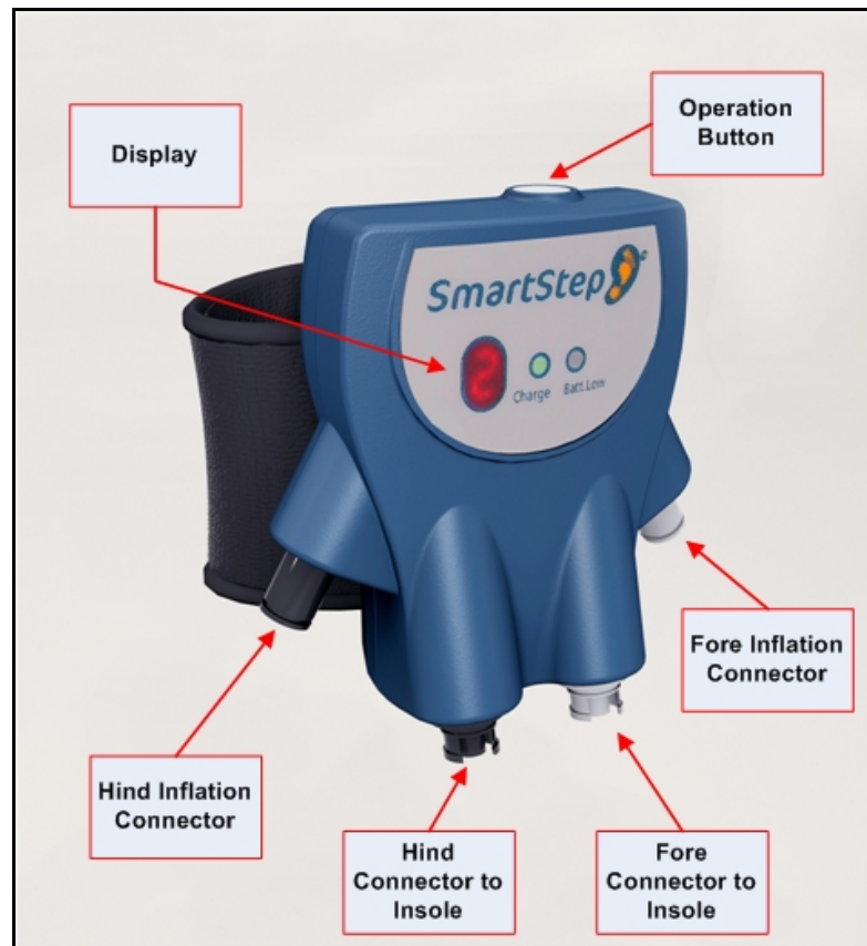
The Control Unit
