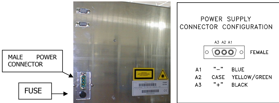
Fig. 27 VDC Connector (TPR922 only)
