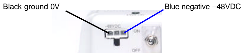
Figure 7 DC Power Connections for Local Unit TFLF
