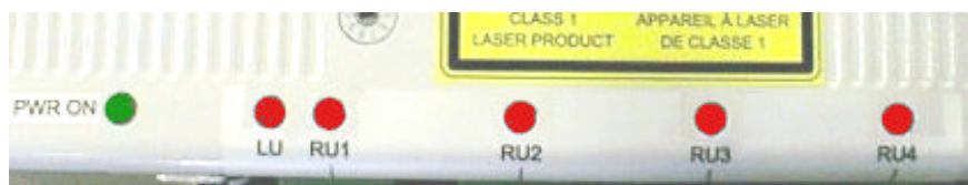
Figure 5 TFLF Local Unit Status LED's
