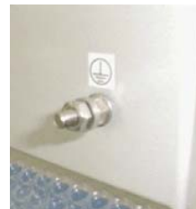
Fig. 14: ground terminal on the rear
