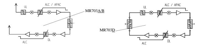
Downlink signals reach the duplexer. The duplexer is the frequency separation unit that splits and recombines uplink (UL) and downlink (DL).
