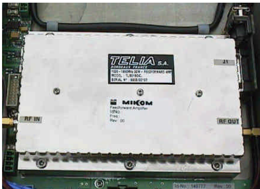
figure 2-9 Top view of the feed forward amplifier
