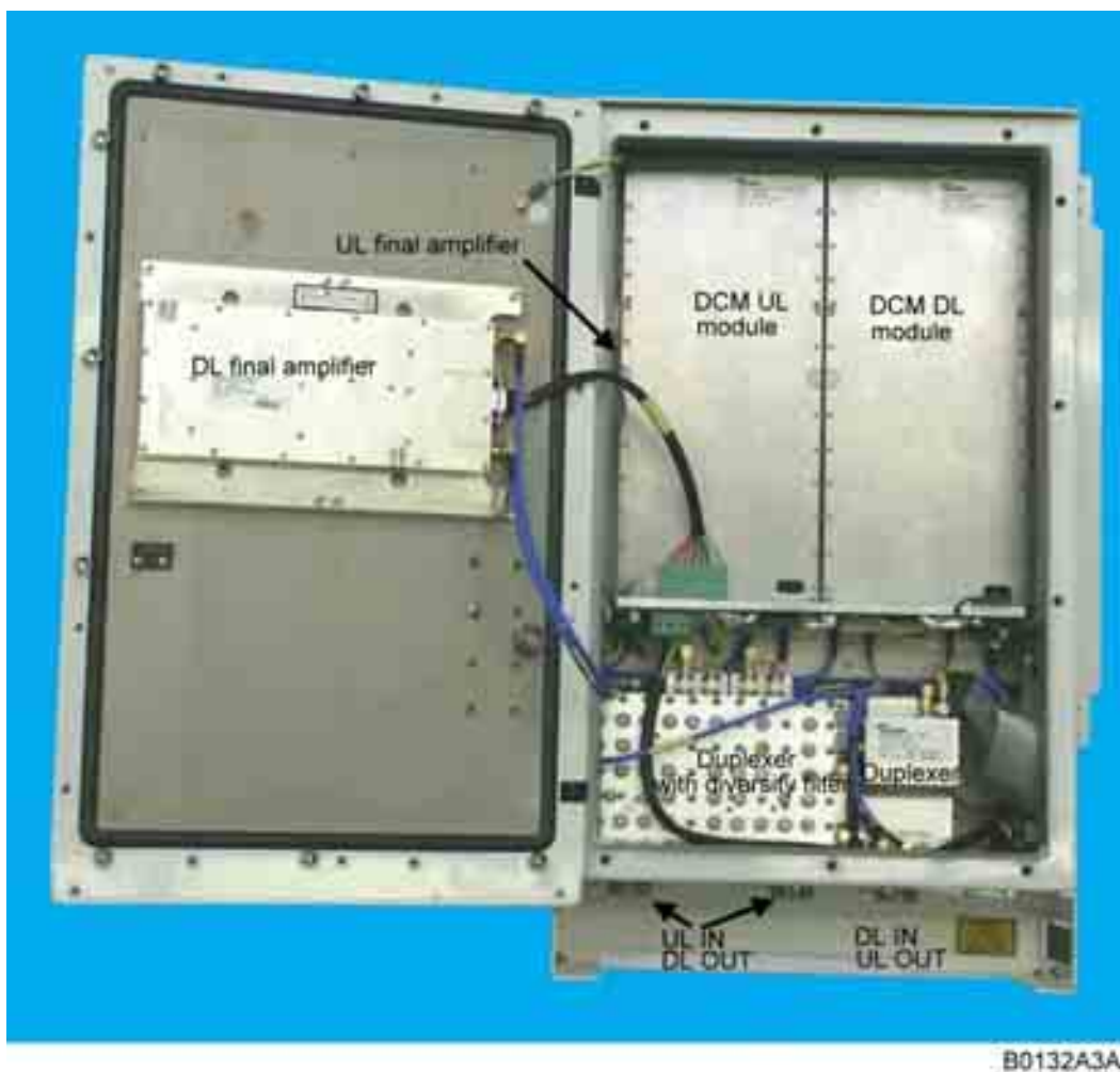
figure 5-3 RF path of a Node C, exemplary
