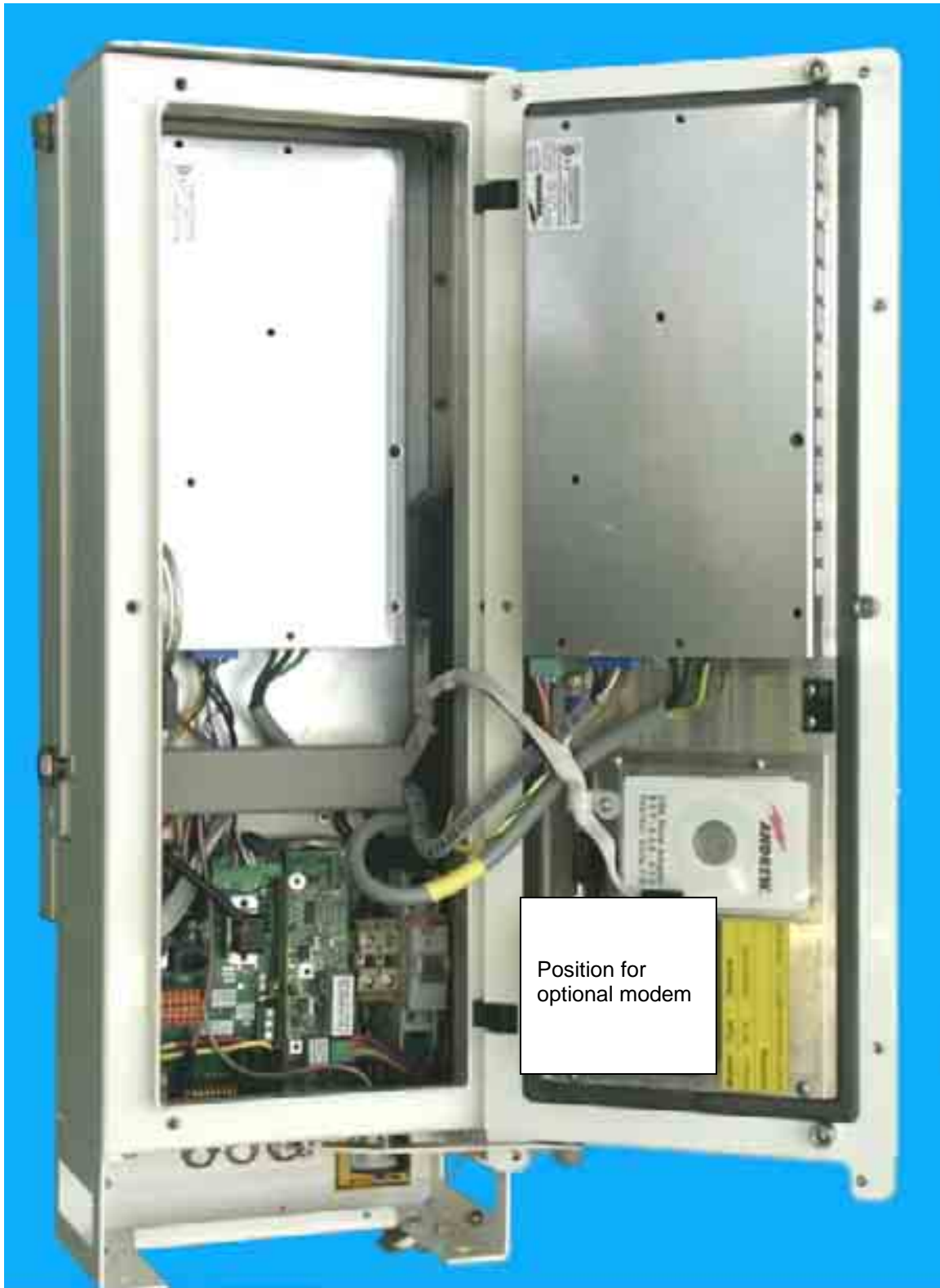
figure 7-5 Layout of the Interface Unit, exemplary
