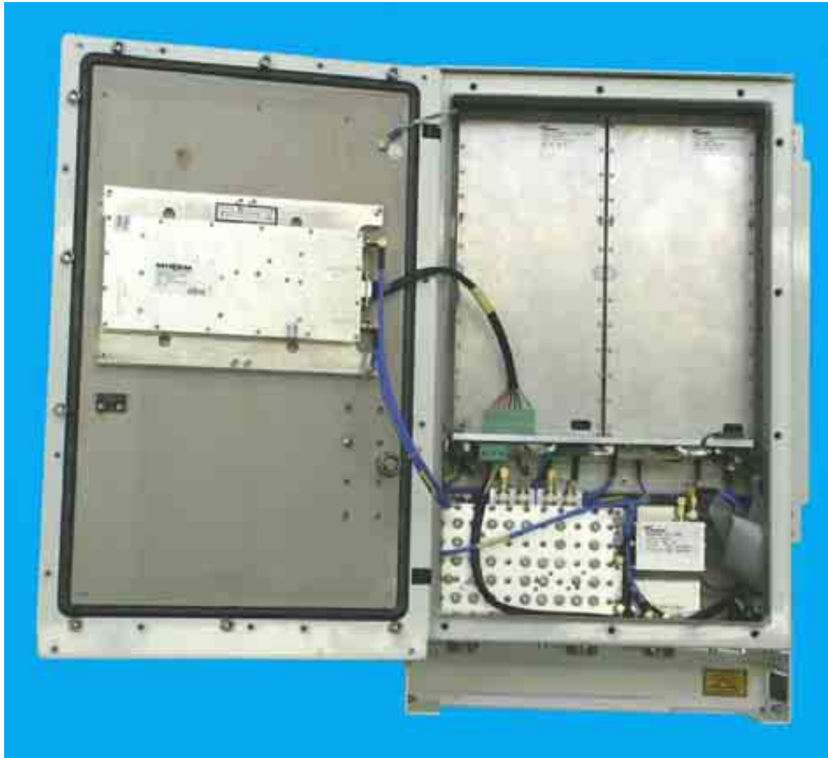
figure 7-3 Layout of the Node C 1937, exemplary
