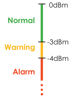
Fig. 3.6.6: AGC thresholds vs LED alerts
