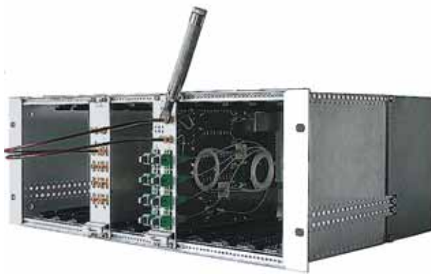
Fig. 4.3.5: Proper cabling of SMA connectors on a TFLN front panel
