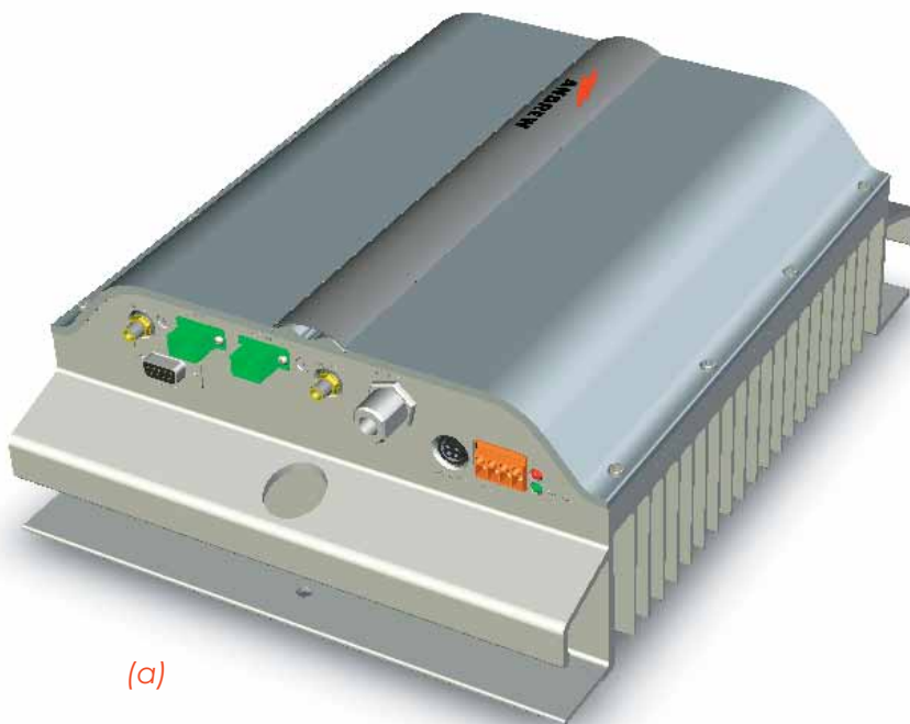
Figure 3.5.1: ION-B, Case-R2 Remote Unit: (a) full view; (b) front view
