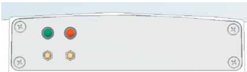
Figure 3.6.2: LED panel on the Case-F Remote Unit
