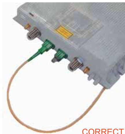
Figure 3.2.5 - Handling optical connections with ION-B Remote Units.
