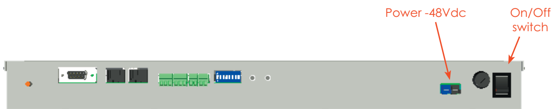
Figure 4.2.3: Rear view of the TPRF31 Fast MiniRack: Power supply connectors and On/Off switches
