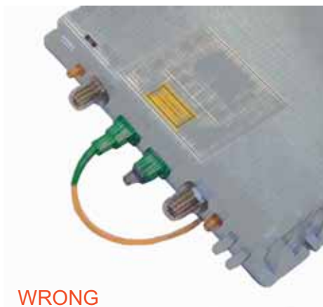
Figure 3.3.5 - Handling optical connections with ION-B Remote Units.
