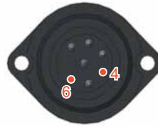
-36/-72 Vdc: Connector 4: 0V 6: -48V
