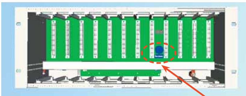
Figure 4.1.7: Dip-switches on the TPRN backplane
