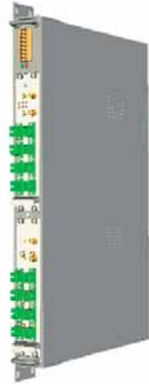
Figure 4.2.12: Wall-mounted TPRF31 Fast MiniRack, hosting 2 TFLNs master unit transceivers
