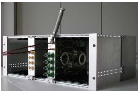
Fig. 5.13: UL and DL RF cables are to be fixed by a torque wrench
