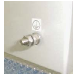
Fig. 5.5: ground terminal on the rear
