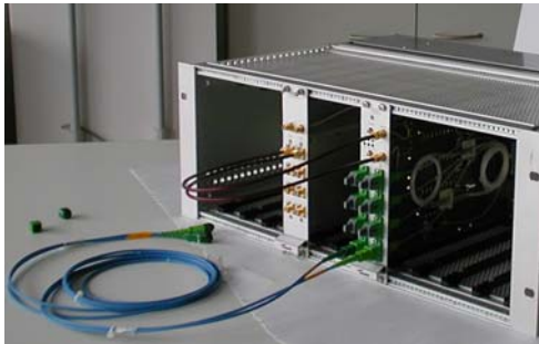
Fig. 5.14: Take off the caps and connect the fiber optics cables properly
