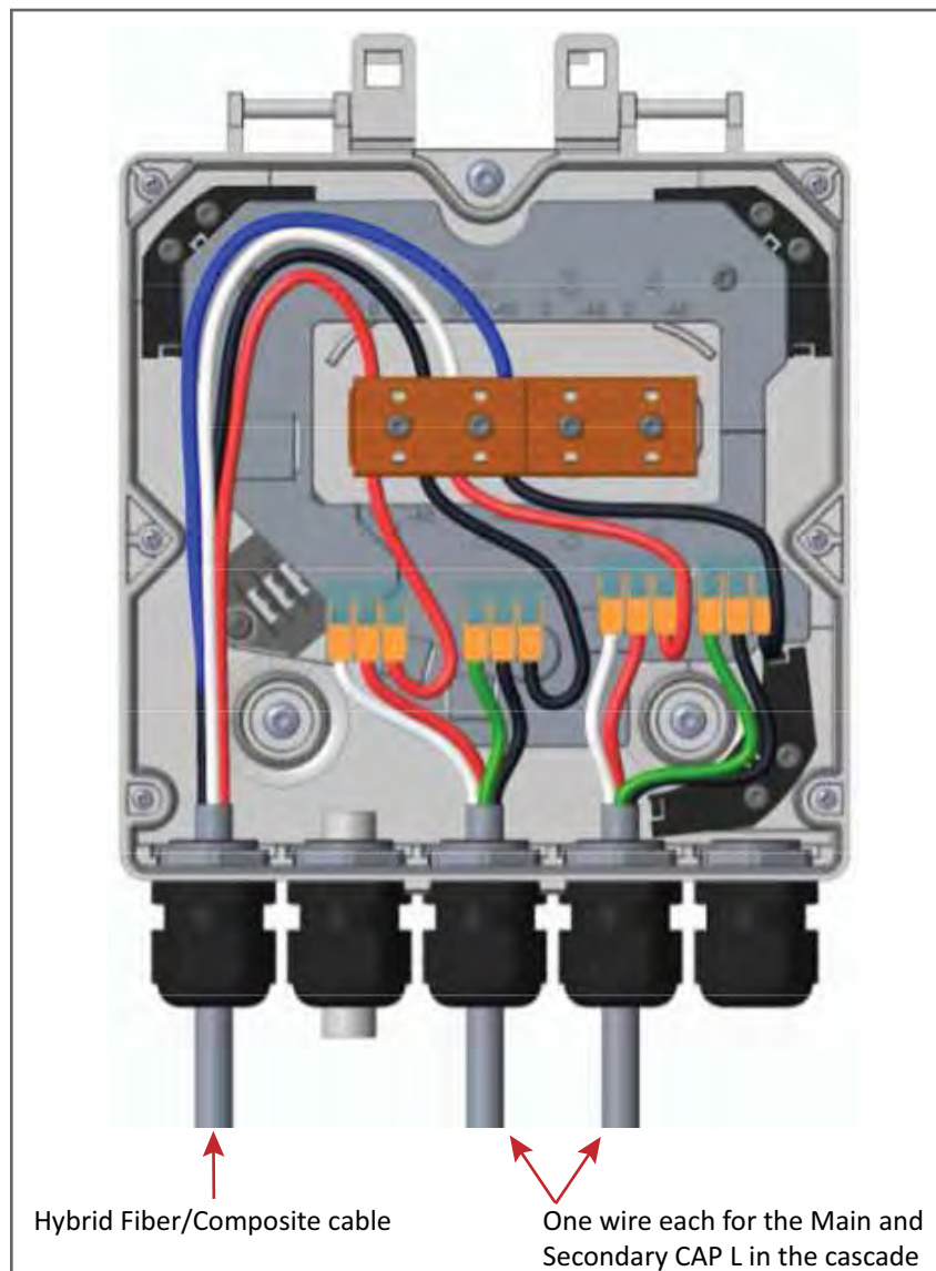
Figure 21. Wiring a Hybrid Fiber Splice Box to Cascade Two CAP Ls in a 2-Wire Power Configuration
