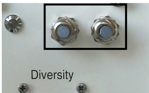
figure 5-22 External cable glands
