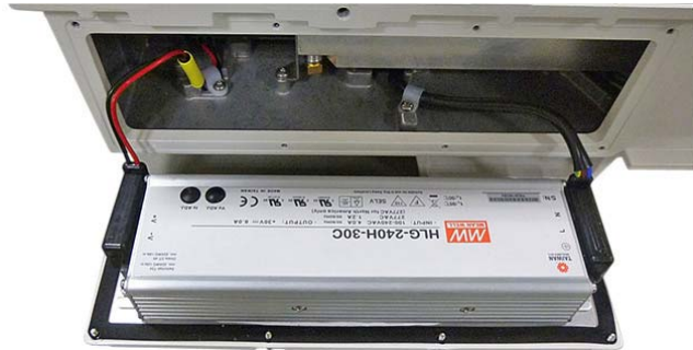
Figure 2-27 RU power supply with cables
