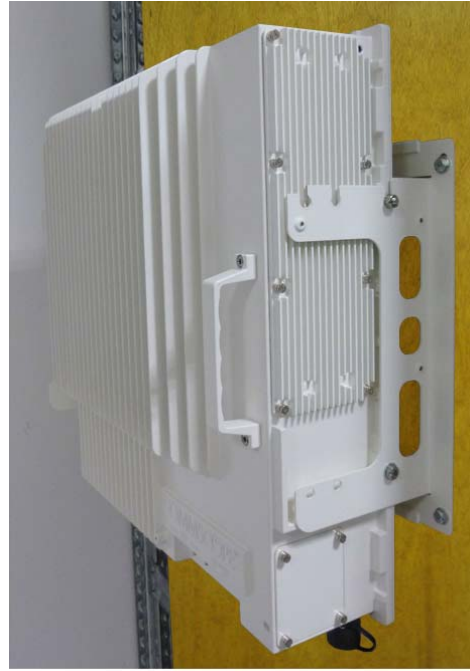
Figure 2-9 Completed RU Mount
