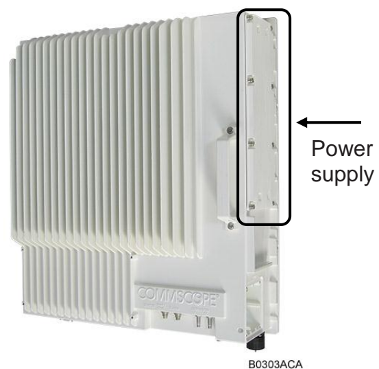
figure 5-2 RU power supply location
