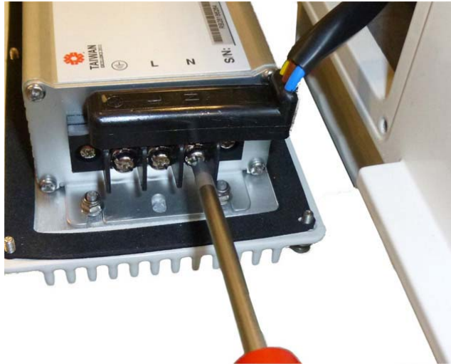
figure 5-5 RU power supply input cable
