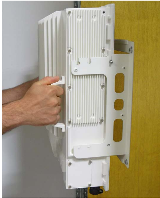
figure 4-6 Place RU onto wall mounting bracket – single mount
