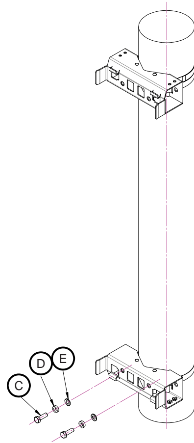
figure 4-5 Pole mounting – fasten EU
