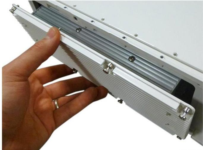
*figure 5-9 EU insert power supply*
