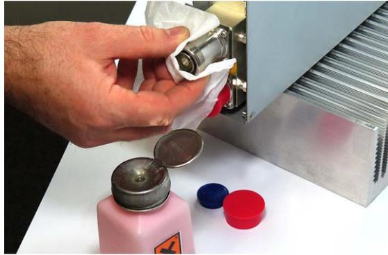
5. Clean the lip of the inner ring with a cotton bud drenched with isopropyl alcohol.
