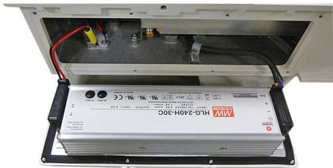
figure 5-4 EU power supply with cables
