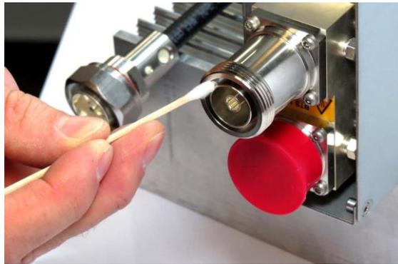
6. Clean the inside surface of the inner ring with a cotton bud drenched with isopropyl alcohol.
