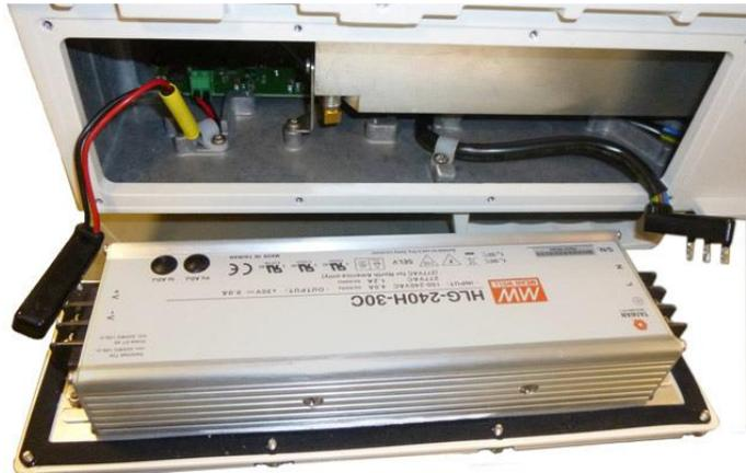
*figure 5-6 EU power supply output cable*
