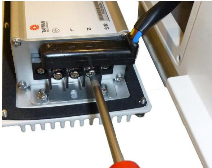
figure 5-5 EU power supply input cable
