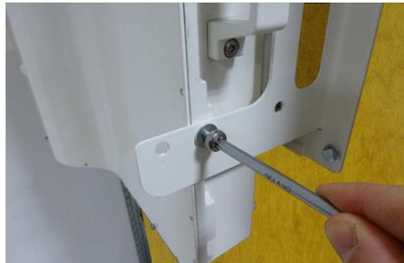
figure 4-11 Install M6x12 screws and washers
