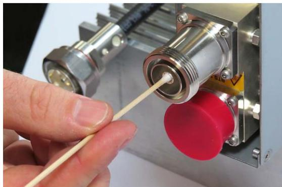
8. Clean in the similar way the connector of the connected cable. Remove protective caps from the unit connector first.
