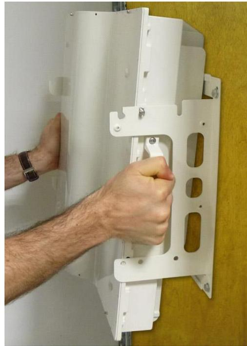
figure 4-10 1<sup>st</sup> unit placed on wall mounting bracket
