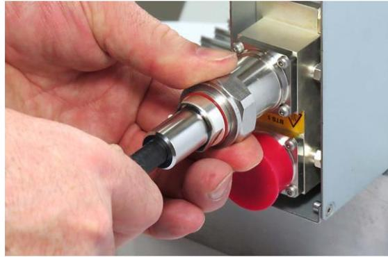
5. Retain the cable connector with the counter wrench and fasten the coupling nut with the torque wrench until the torque is applied (torque wrench clicks).
