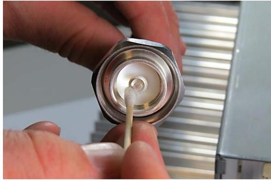
**4.2.6.2. Antenna cable connector assembly**
