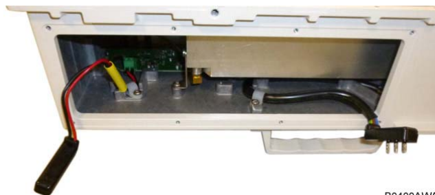
figure 5-7 EU with power supply removed
