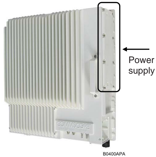
figure 5-2 EU power supply location
