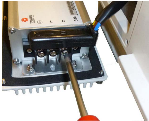
figure 5-5 EU power supply input cable
