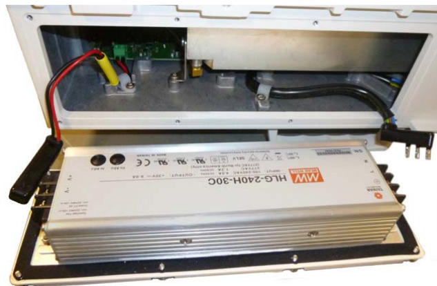
figure 5-6 EU power supply output cable
