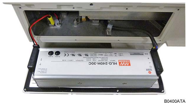
figure 5-4 EU power supply with cables
