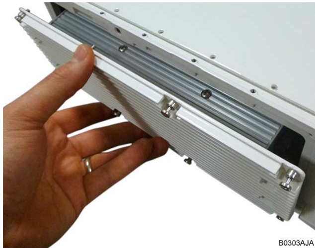
figure 5-9 EU insert power supply
