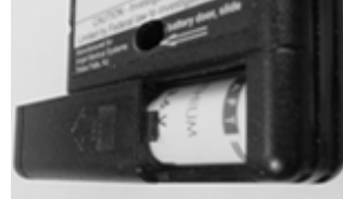
Fig. 11a – d. Replacing the Battery
