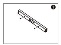
Step 2: Place the wall mounting template against the wall, under your TV. Mark the 4 bracket holes on the wall with a pencil.
