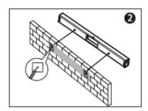
Step 3: Fix the two mounting brackets on the wall according to the center points. Use bolts (not included) to secure the brackets.
