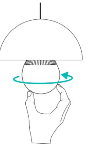
Make sure the power switch controlling Lumos is turned off before installing.
