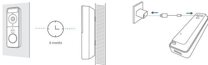
**Note:** The battery life varies depending on usage. In most common cases, a doorbell may have up to 15 events per day and each recording lasts 20 seconds on average. Under this scenario, the doorbell battery life can last up to 4 months.
