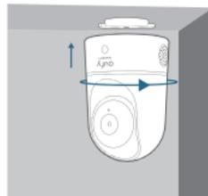
To mount the Indoor Cam on a wall, we recommend using the mounting bracket (not provided) as the illustration below.
