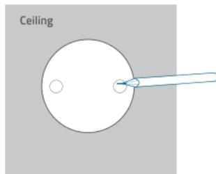
2. Drill holes with a 5/16" (8 mm) drill bit.
