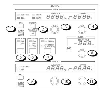
1 Termination conditions setting (DATA side) DATA/DATA displaying switching and DATA/DATA tracking Amplitude (DATA side) Offset (DATA side) 5 Output ON/OFF 6 Offset display standard setting 7 1/1 SPEED / 1/4 SPEED display switching 8 CLOCK delay 9 Termination conditions setting (CLOCK 1 side) 10 Amplitude (CLOCK 1 side) 11 Offset (CLOCK 1 side)
