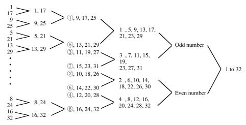
The numbers in circles  $(\bigcirc)$  indicate the output order for 1/8 DATA OUT.
