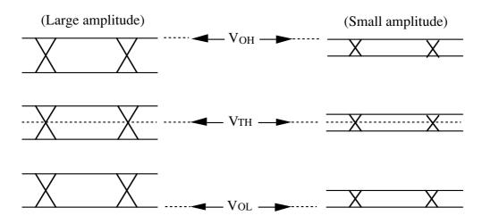
Fig. 4.3.5-1 Offset Reference Value and Amplitude Change
