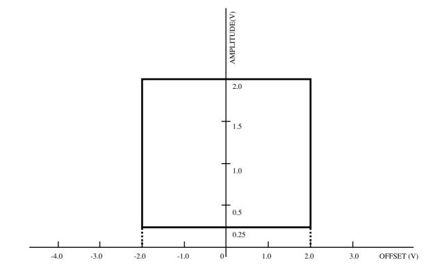
Fig. 4.3.5-2 Amplitude and Offset Voltage Setting Range Corresponding to Offset Reference Value
