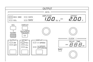
When the setting of ④ is changed, the actual waveform and output do not change. Only the displayed value changes (see the figure below).
