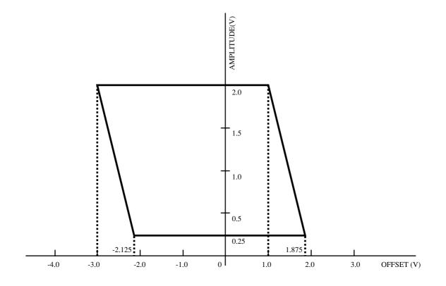
Fig. 4.3.5-3 Amplitude and Offset Voltage Setting Range Corresponding to Offset Reference Value
