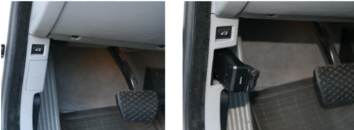
Figure 4.1: Installation of ACT233L in vehicle
