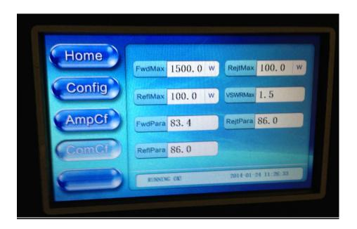
**<u>PreAmpCf Screen</u>**: This screen is used to configure the Premap maimum operating thresholds to engage safety and protective power reduction and shutdown mechanisms.
