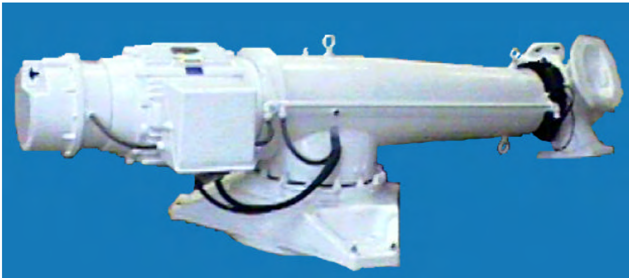
Figure 2-3 AOC 15/50 Drive train assembly
