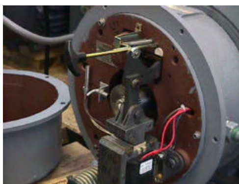
Figure 12.1-4 Stearns parking brake with speed pickup and temperature sensor
