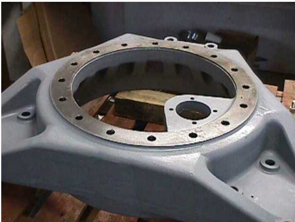
Figure 6-6 Tower top casting
