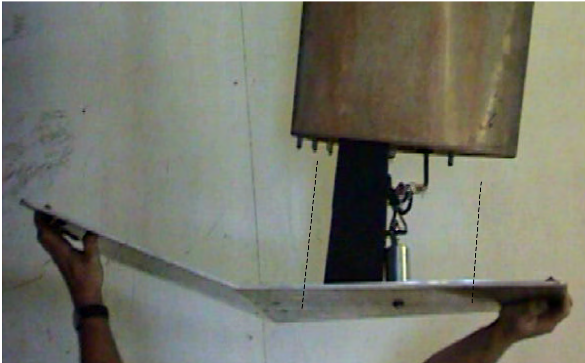
Figure 6-2 Tip brake installation
