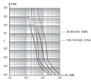
UPS short-circuit current with inverter coupled and By-pass AC source out of tolerances
