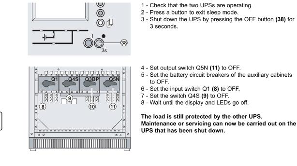
Figure 4-3: Parallel UPS Configuration Without External Bypass Cabinet
