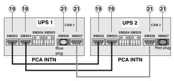
**Exchange-current interconnections (19):** Link connectors XMS02 and XMS03 on the two UPS units.
