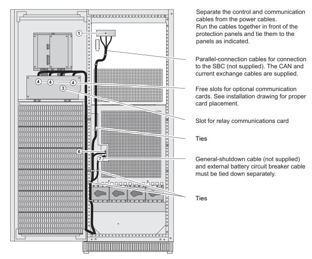
Figure 2-15: Routing the Control/Communications Cables for Parallel UPS
