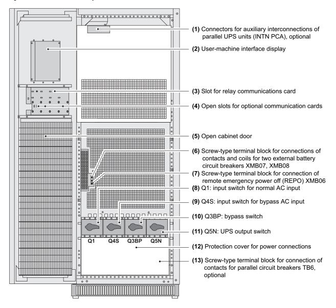
Figure 1-4: Power Connection Terminals
