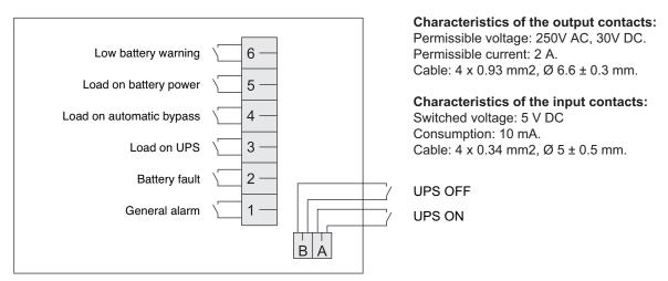
Figure 2-13: Characteristics of the Contacts on the Relay Communications Card
