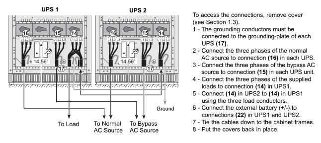
If the two UPSs are placed side by side, connect as indicated above. In the other configurations, always make sure that the cables between the UPSs and bypass AC source have the same cross-section and the same length. The same is true for the cables between the UPSs and the load.
