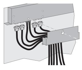
Note: Tie down the cables as indicated in the diagram in Section 2.9.
