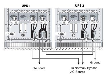
Figure 2-5: Parallel UPS With Common Normal and Bypass AC Inputs
