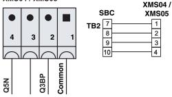
**Note:** The interconnection cables for the SBC are not supplied
