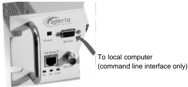
Figure4-7 Connecting to the RS-232 Craft Port
