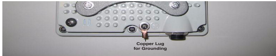
Figure 2-10 Location of Grounding Lug on Outdoor Unit (Radio/Antenna)
