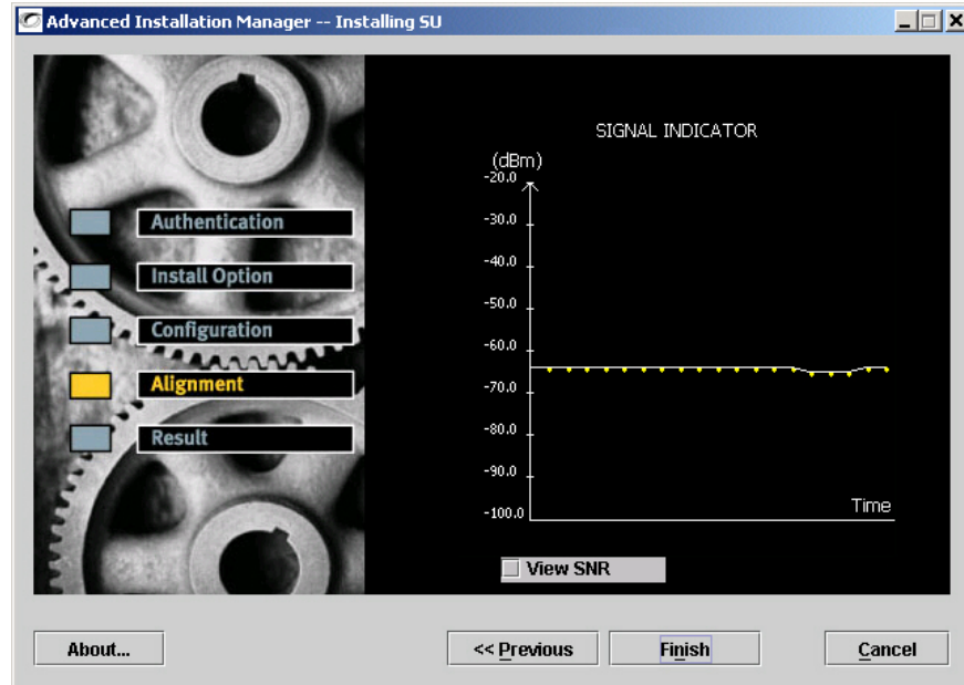
Figure 2-10 Alignment Window of PW610 - First Step
