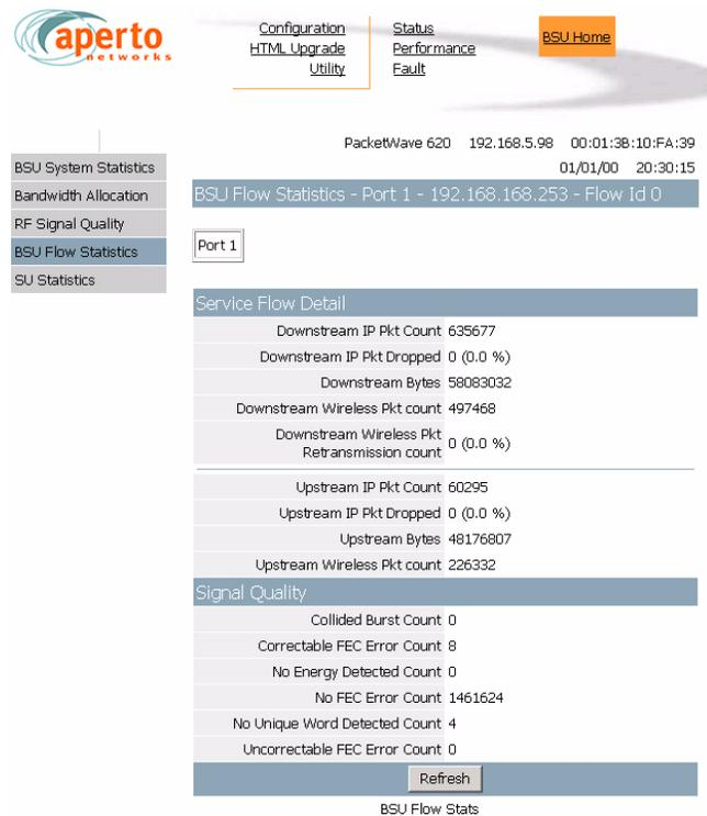
**Figure 3-22 BSU Flow Statistics by Flow ID**
