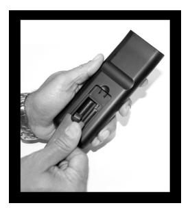
• To insert batteries, turn the remote control over and remove the battery cover.
