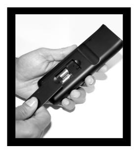
• Place two (2) AAA batteries into the compartment with correct polarity.
