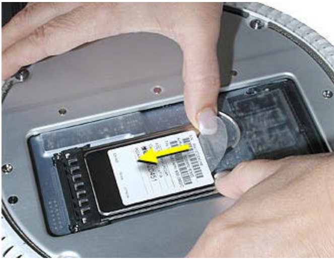
Figure 7 Insert the card into the slot
