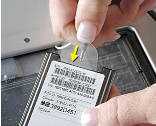
Figure 6 Insert the antenna to connect it
