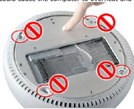
Figure 5 Do not remove these screws
