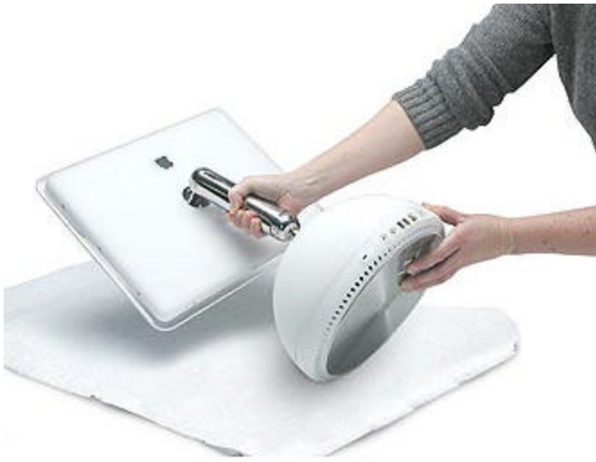
Figure 2 Lay down the computer
