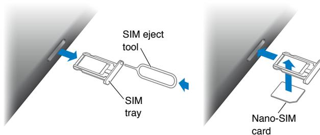
**Open the SIM tray.** Insert a SIM eject tool (sold separately) into the hole on the SIM tray, then press firmly and push the tool straight in until the tray pops out. Pull out the SIM tray to install or replace the SIM card. If you don't have a SIM eject tool, try the end of a small paper clip.
