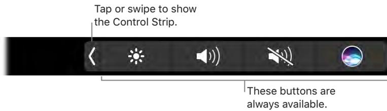
**Open or close the Control Strip.** Frequently used system controls, like volume and brightness, are located in the Control Strip on the right side of the Touch Bar. (These functions are described in [Keyboard](#).) Tap or swipe to expand the strip, tap buttons or sliders for the settings you want to change, then tap Done when you finish. Or leave the Control Strip open to keep those buttons available.
