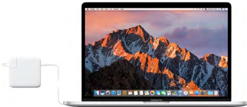
**Charge the battery.** Connect your MacBook Pro to a power outlet using the included USB-C Charge Cable and 61W or 87W USB-C Power Adapter. You hear and may feel a vibration when you connect. The battery recharges more quickly when the computer is off or in sleep.
