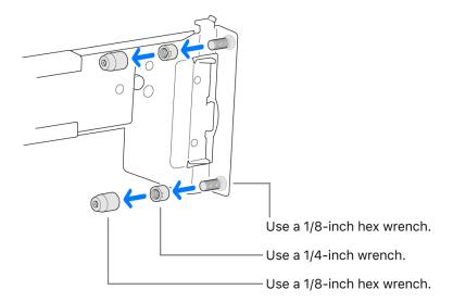
To install Mac Pro into a rack, you need to attach the rail assemblies to Mac Pro and the rack. The minimum depth of the rack must be at least 24 inches; the maximum depth should be no more than 42 inches.
