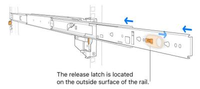
2. Push in the rear orange latch at the back of the rail, then push the assembly back to unhook the rear pins.
