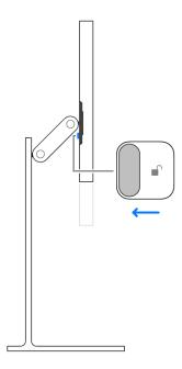
3. Rotate the display counterclockwise. When it reaches portrait orientation, the display automatically locks.
