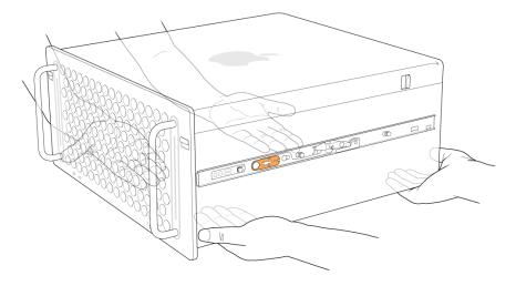
4. Pull the orange release latches on both rails, then remove Mac Pro from the rack.
