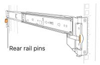
3. Insert the assembly's front rail pins into the front of the rack, then push the assembly to lock it into place.
