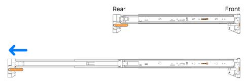
2. Insert the assembly's rear rail pins into the back of the rack, then pull the assembly to lock it into place.
