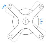
4. Use the key provided to turn the lock clockwise to secure the adapter.
