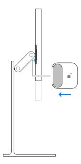
3. Tilt the display back and lift it from the magnetic connector.
