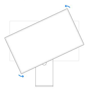
4. To rotate to landscape orientation, repeat step 2, then rotate the display clockwise.
