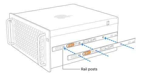
8. Slide the rail section forward until the spring lock engages the forward post.
