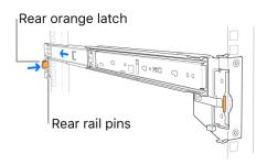
3. Open the latch at the front of the assembly to release the front pins, then lift the assembly out of the rack.
