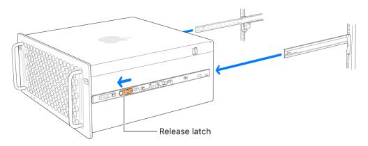
*Note:* You can detach the rails from the side of Mac Pro by pulling the spring latch forward, then sliding the rail back.
