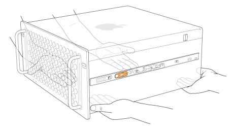
10. Align the rails attached to Mac Pro with the middle rails in the rack, then slide the computer into the rack. Ensure the locking latches are fully engaged.
