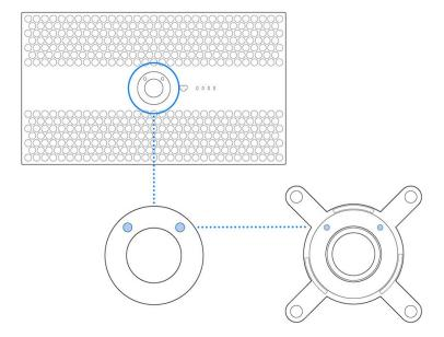
3. Place the adapter and rotate slightly in either direction until the pins click into place. The lock will be in the vertical position.
