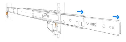
5. Slide the release latch to detach the inner rail from the assembly.
