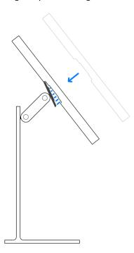
2. Lower the display onto the connector. When close, the display magnetically attaches to the stand. If placed correctly, the display locks into place.
