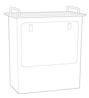
6. Push in the top of the latches, then pull the latches to remove the access door.
