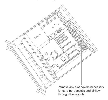
11. Push the ejection arm on the new module, then push the module into place.
