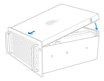
**WARNING:** Do not try to operate Mac Pro with the cover removed as interlock circuitry will prevent the computer from starting up. Do not defeat the purpose of the interlock circuitry—it protects you from the fan blades and hazardous energy on the motherboard.
