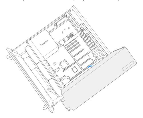
12. Slide the PCI retention latch (numbered 2) to the left.
