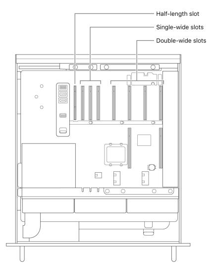
**WARNING:** For optimum ventilation, space cards out as you install them. If you remove a card and don't install a replacement, place a port access cover over the empty slot to keep foreign objects out of the enclosure. An uncovered slot affects the airflow that cools the internal components, and may cause damage.
