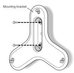
**3** Locate the two mounting bracket holes on the bottom of the base station.
