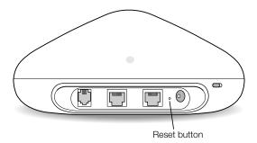
The middle light flashes, indicating that the base station is in reset mode. The base station remains in reset mode for five minutes. If you do not make your changes within five minutes of pressing the reset button, you must reset it again.
