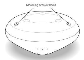
Feed the cables through the mounting bracket and then connect them to the base station.
