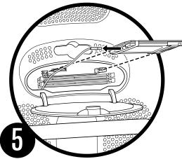
Align the edges of the AirPort Card adapter (which holds the AirPort Card) with the guides on the slot and insert it sideways into the slot.
