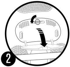
Unlock the access door using a coin, then open the door.
