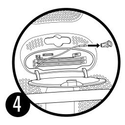
Detach the antenna from the left rail guide on the upper AirPort Card slot and remove the protective cap. Then connect the antenna to the AirPort Card.
