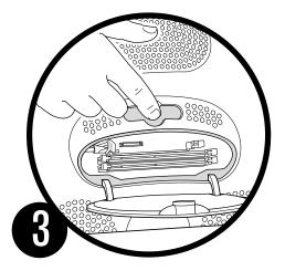
Touch the metal shield inside the recessed latch area to discharge static electricity. Then unplug the power cord from the computer.
