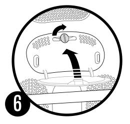
Close the access door and use a coin to lock it. Reconnect all cables and cords, then press the Power button on the computer.
